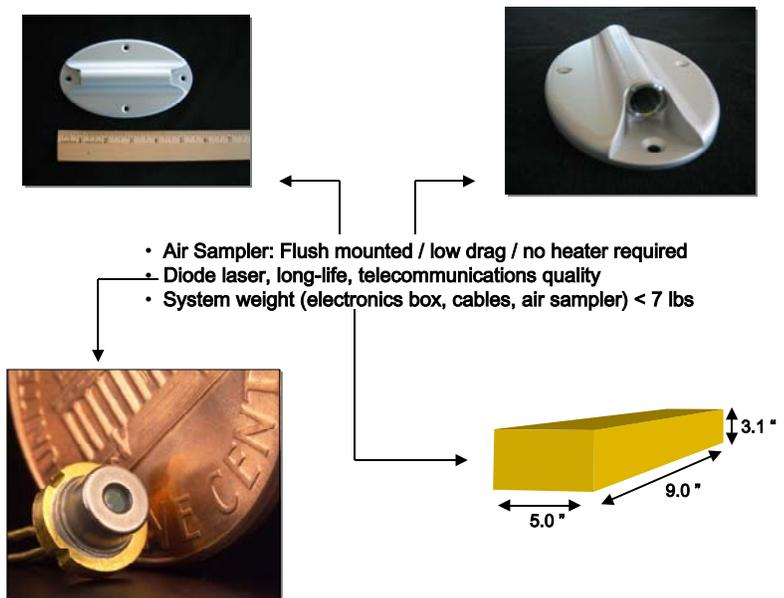
**Figure 7:** Composite of WVSS-II components
