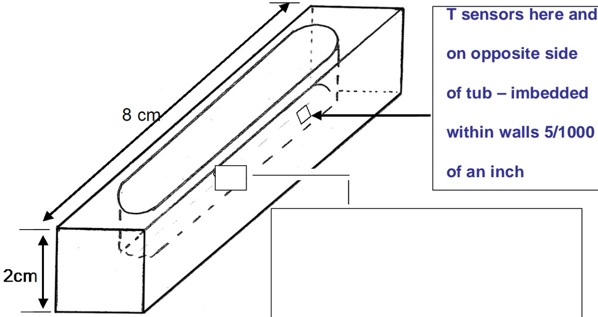
T sensors here and on opposite side of tub – imbedded within walls 5/1000 of an inch
